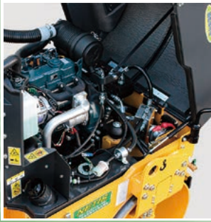
Full open type engine hood with noise absorber
