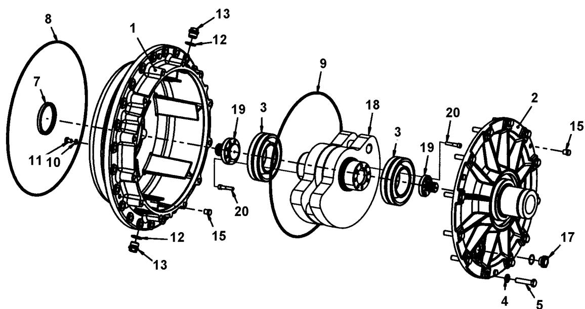
**4812158090 Drum cartridge, vibration side (PD version)**
