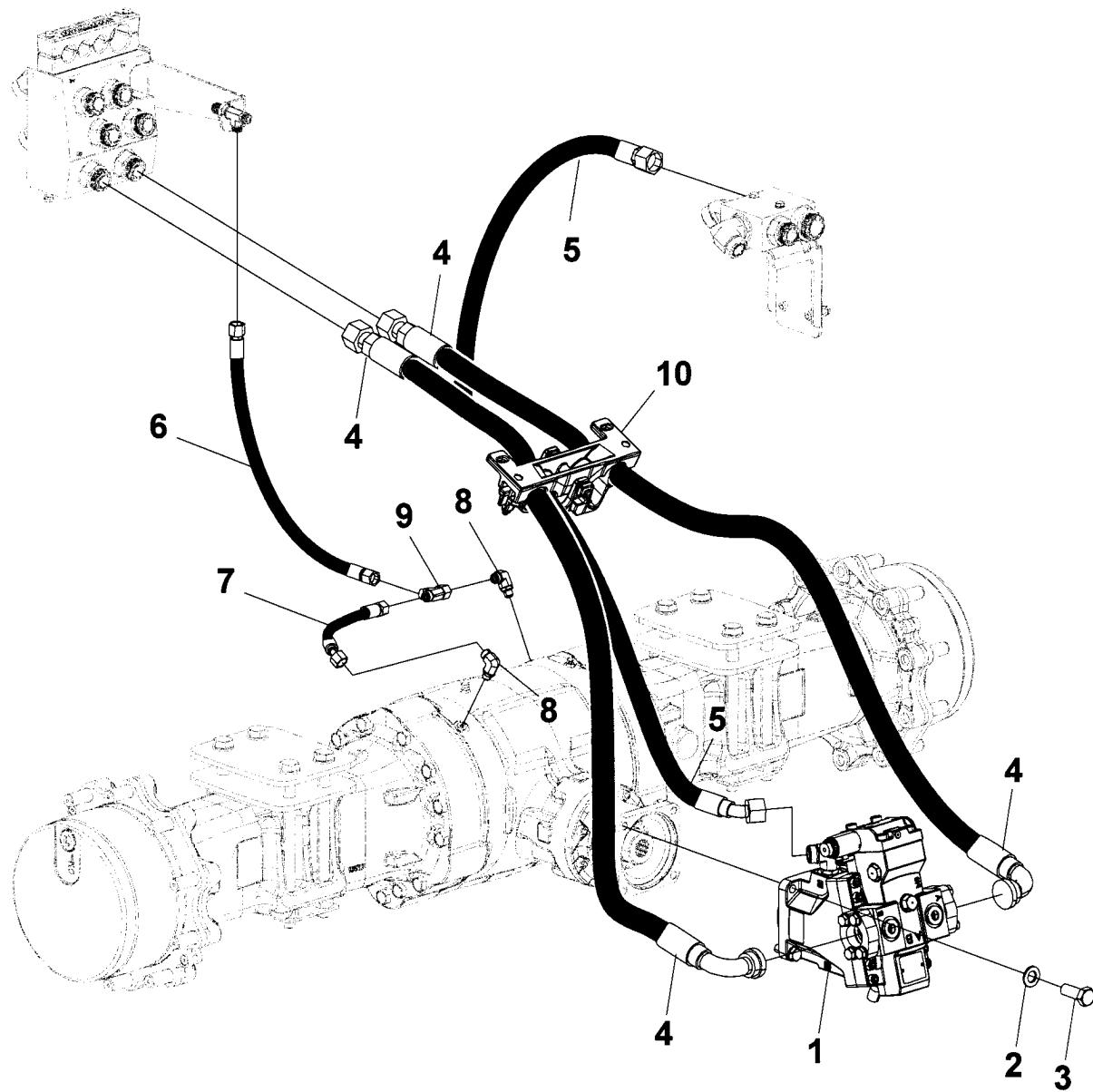
**Hydraulic system, rear axle Traction control, limited slip**
