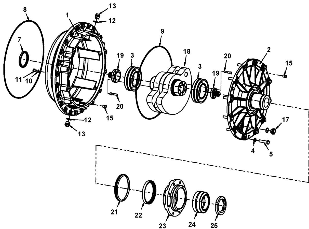
**4812158095 Drum cartridge with shaft nut, vibration side (PD version)**
