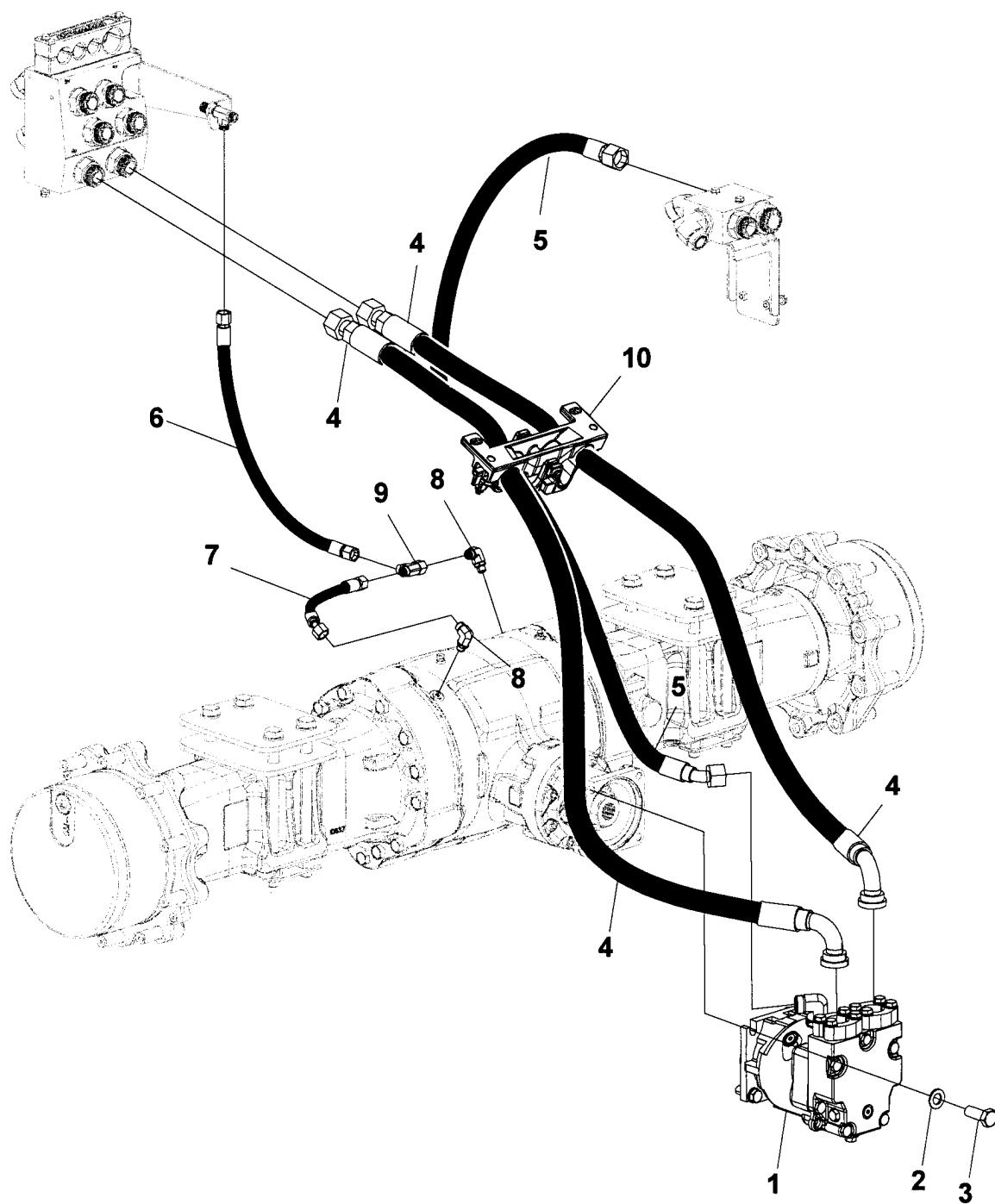
**Hydraulic system, rear axle Dual speed**
