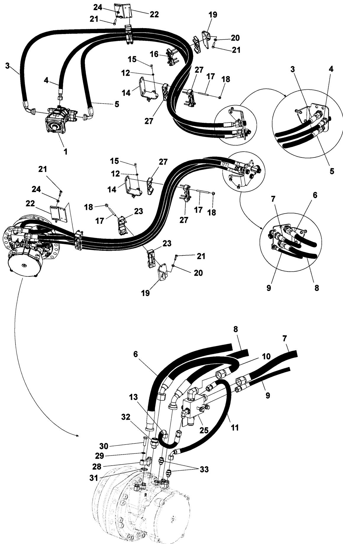
**Hydraulic system, drum (D) Traction control, dual speed**
