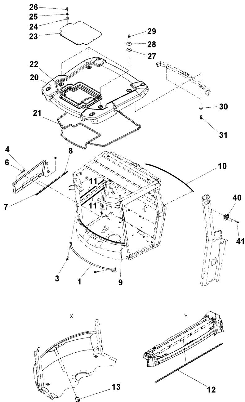
**Basic kit Rops, roof, front handrail**
