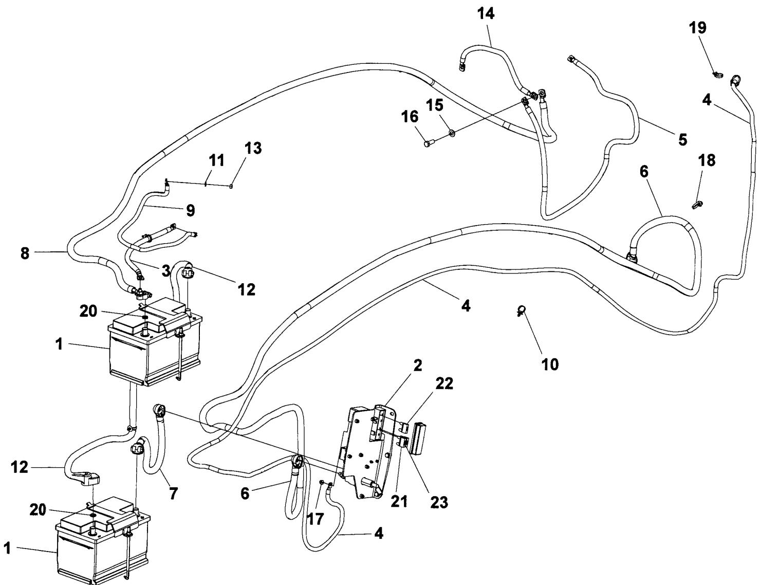
**Electric cables, power supply, 1-pole**
