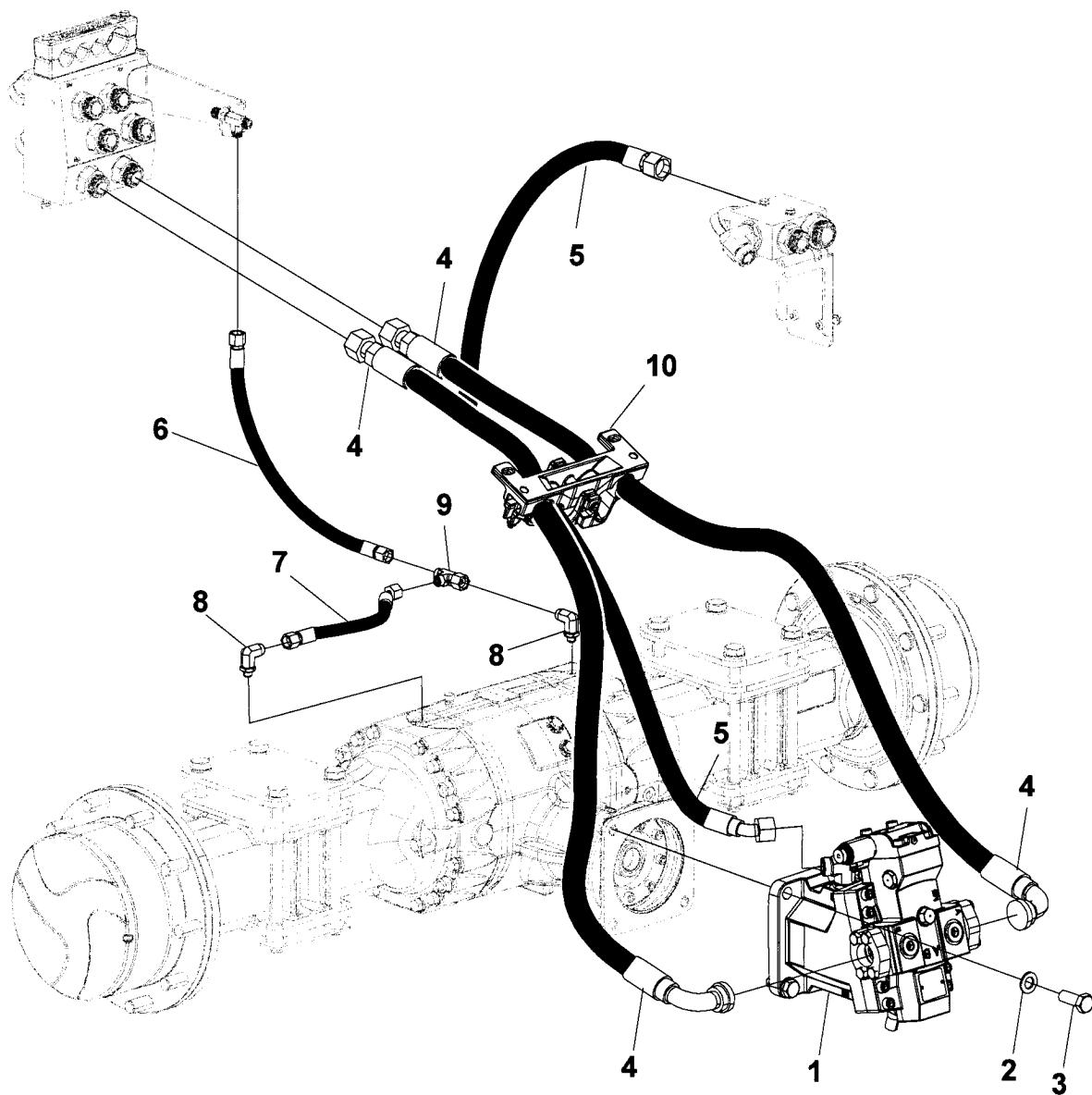
**Hydraulic system, rear axle Traction control, no slip**
