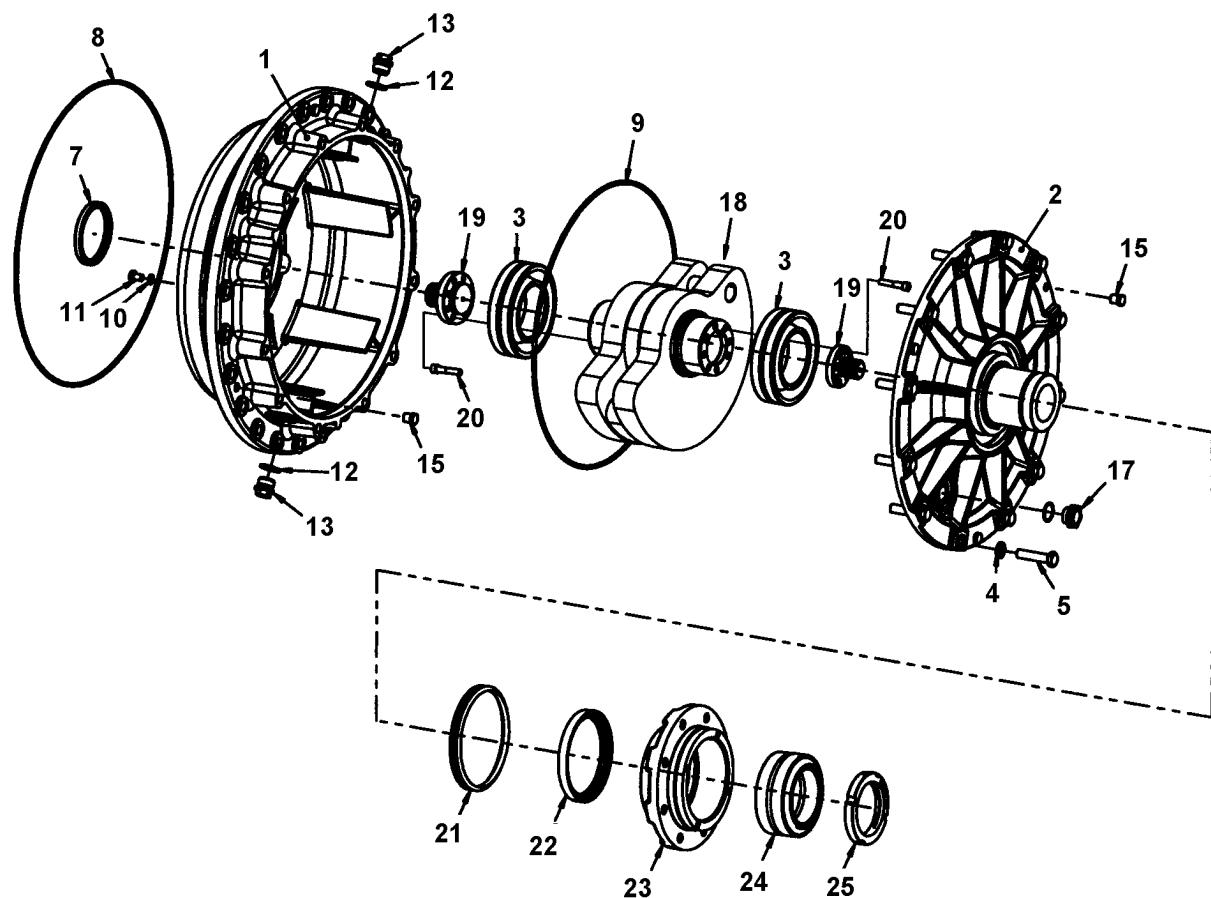
**4812158096 Drum cartridge with shaft nut, vibration side (D version)**
