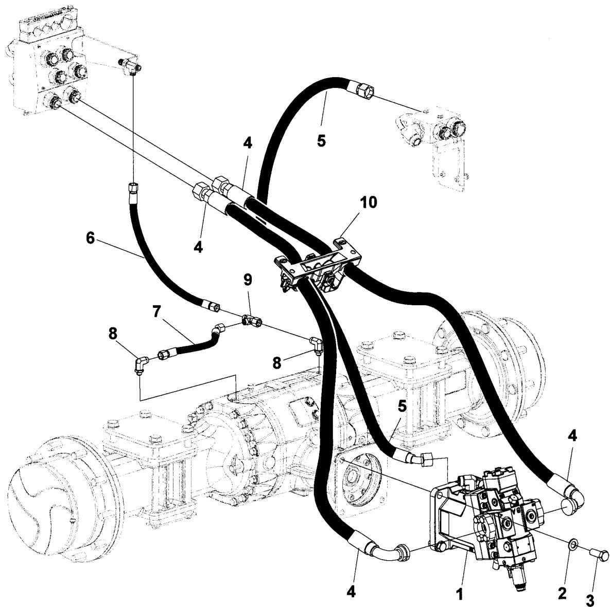
**Hydraulic system, rear axle Anti-spin system**
