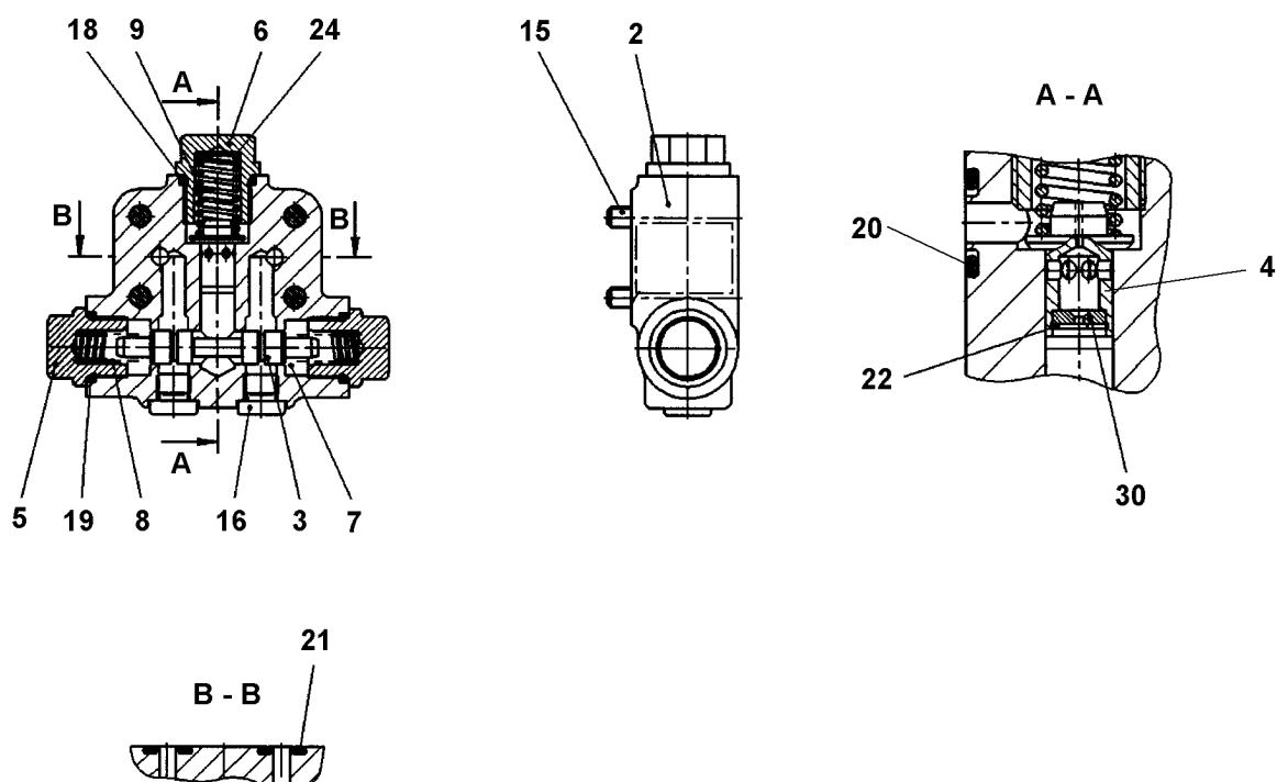
**Flush & boost pressure valve with orifice**
