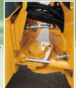
Articulated steering system with oscillation function
